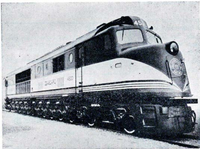
Seaboard-Airline-Railway, Norfolk, U.S.A., 3000 hk diesel el-loko
