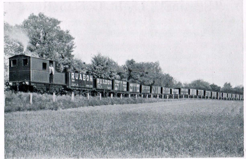
12-Ton Locomotive Hauling 20 10-Ton Waggons
