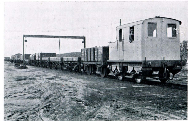
20-Ton Locomotive Exerting a Drawbar Pull at Starting of 5\frac{1}{2} Tons on Dry Rails
