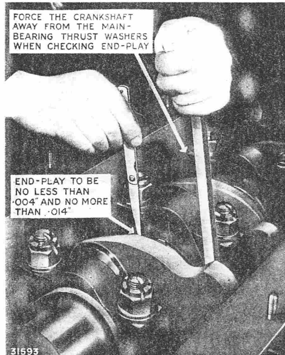
FIG. 76. CHECKING CRANKSHAFT END PLAY
