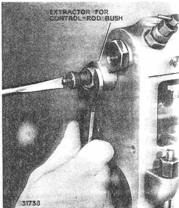
FIG. 34. REMOVING CONTROL ROD BUSHES
