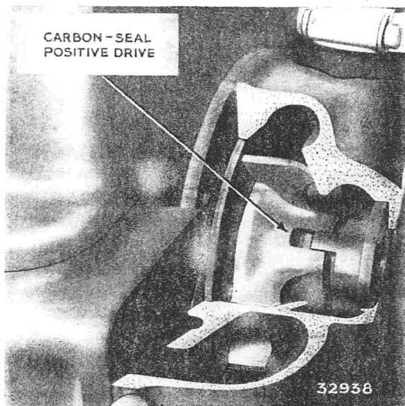
FIG. 101. WATER-PUMP CARBON-SEAL POSITIVE DRIVE
