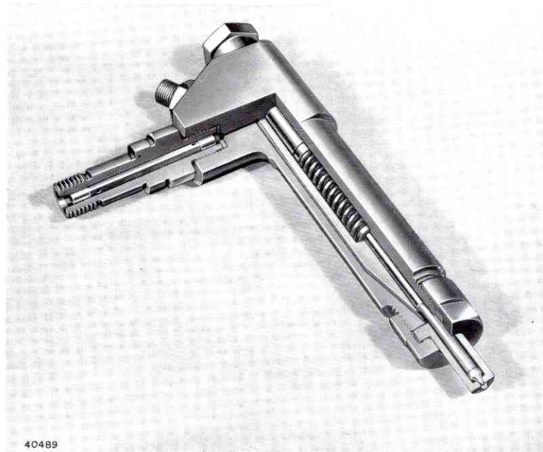
FIG. 46. AN INJECTOR UNIT SECTIONED
