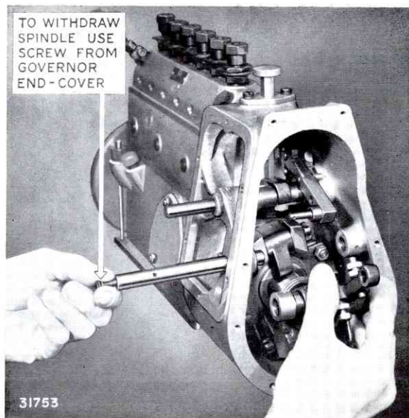
FIG. 82. REMOVING GOVERNOR LINKAGE
