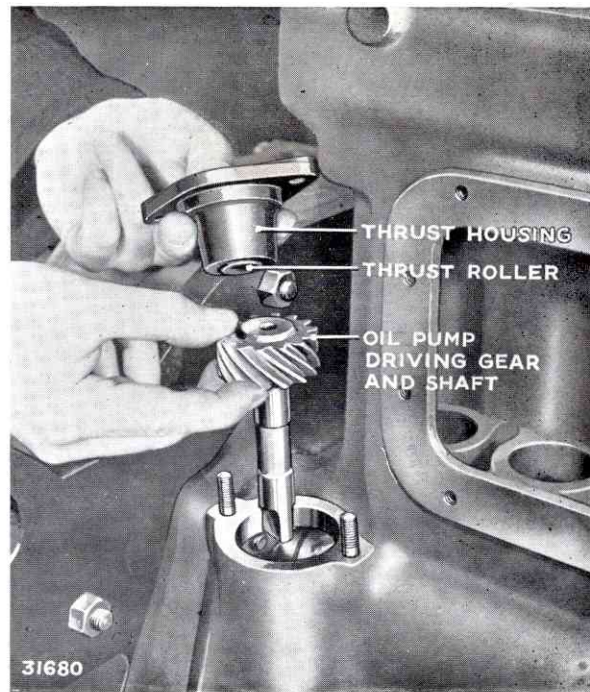
FIG. 9. FITTING OIL PUMP DRIVE GEAR AND THRUST HOUSING
